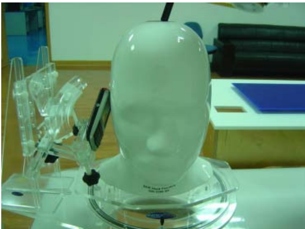
Fig.6 EUT Right Head Tilt15 Position
