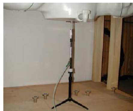
Figure 12.1 Dipole Validation Test Setup
