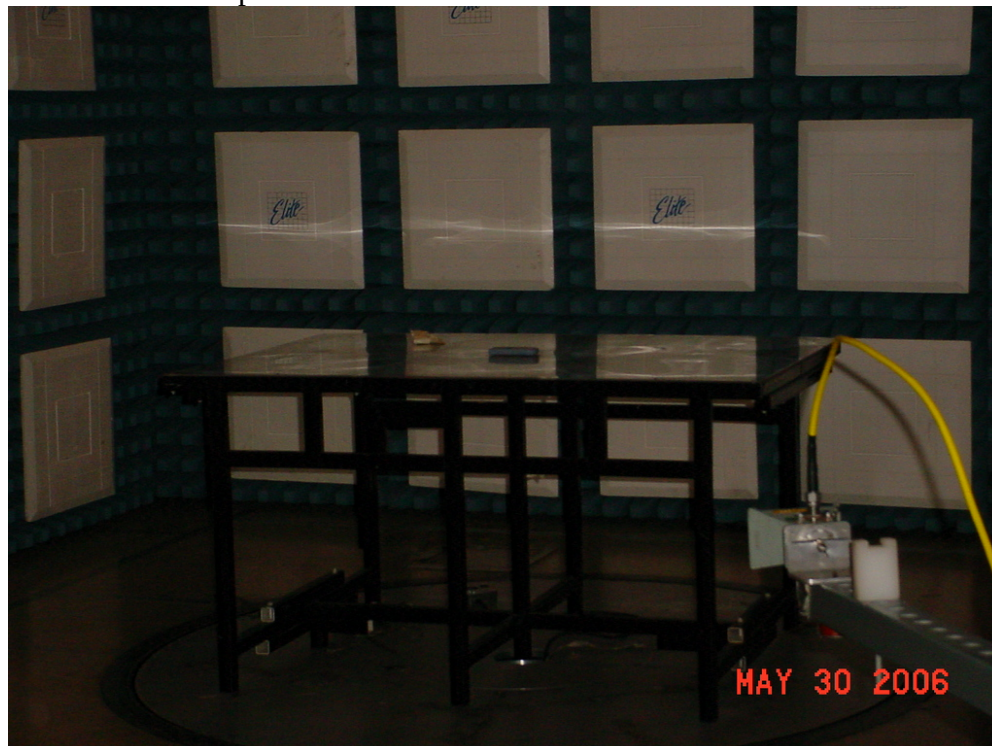
Test Setup for Radiated Emissions – Vertical Polarization
