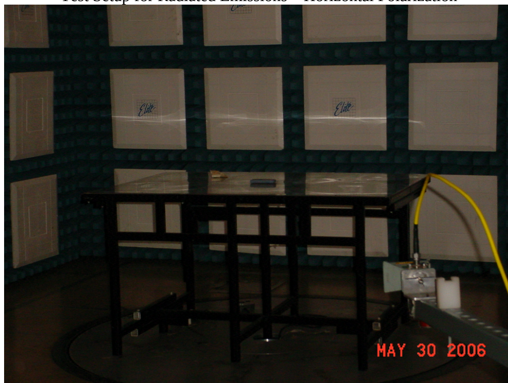
Test Setup for Radiated Emissions – Vertical Polarization
