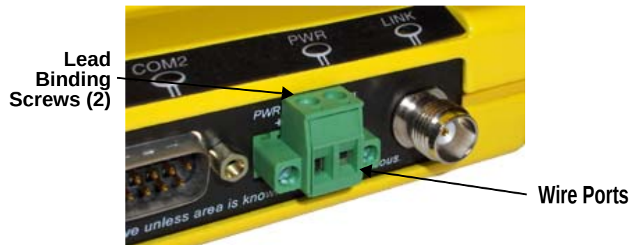
Figure 2-2. Power Connector, Polarity: Left +, Right –
