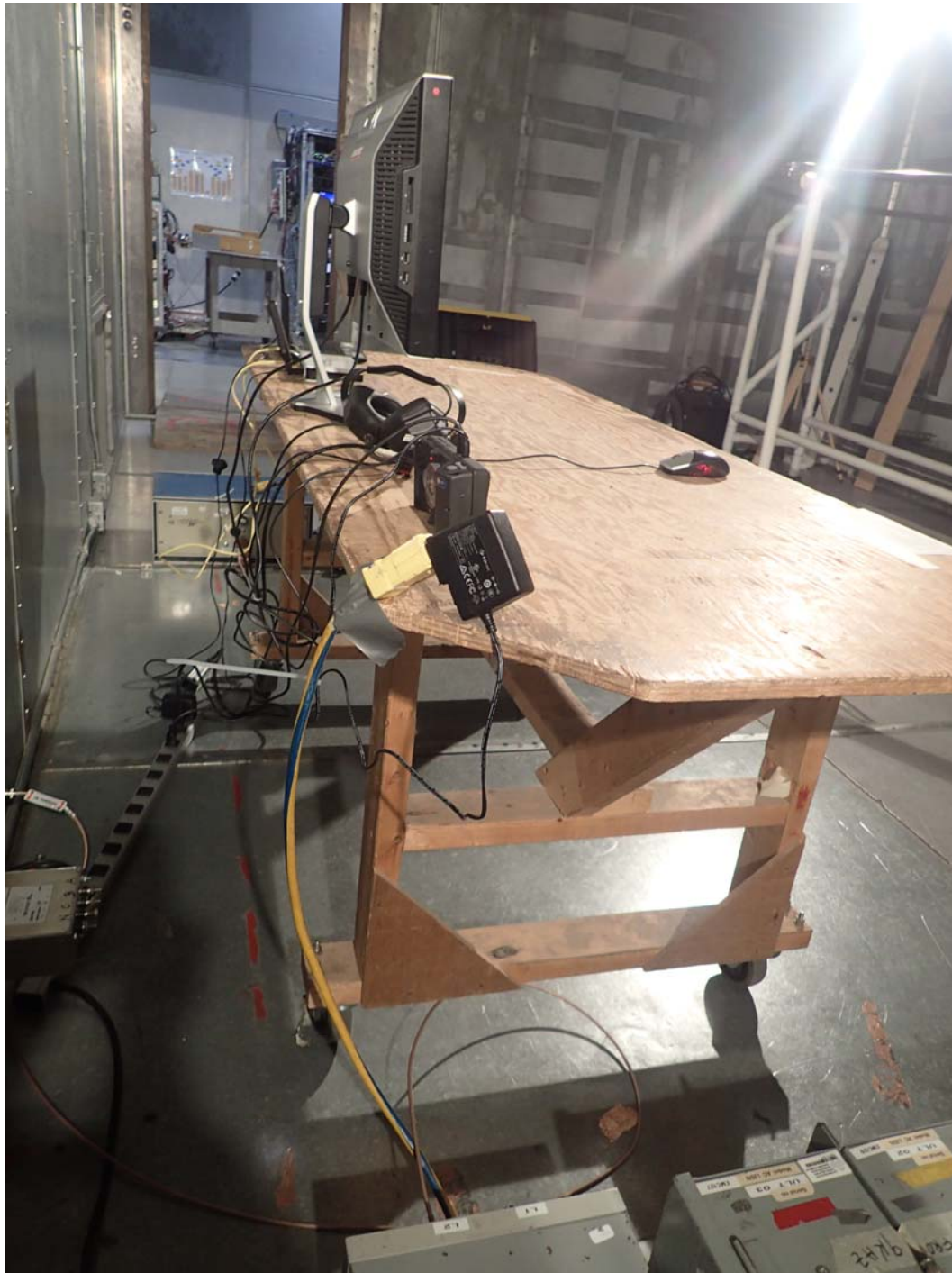
Power Line Conducted Emission (without aluminum shield)
