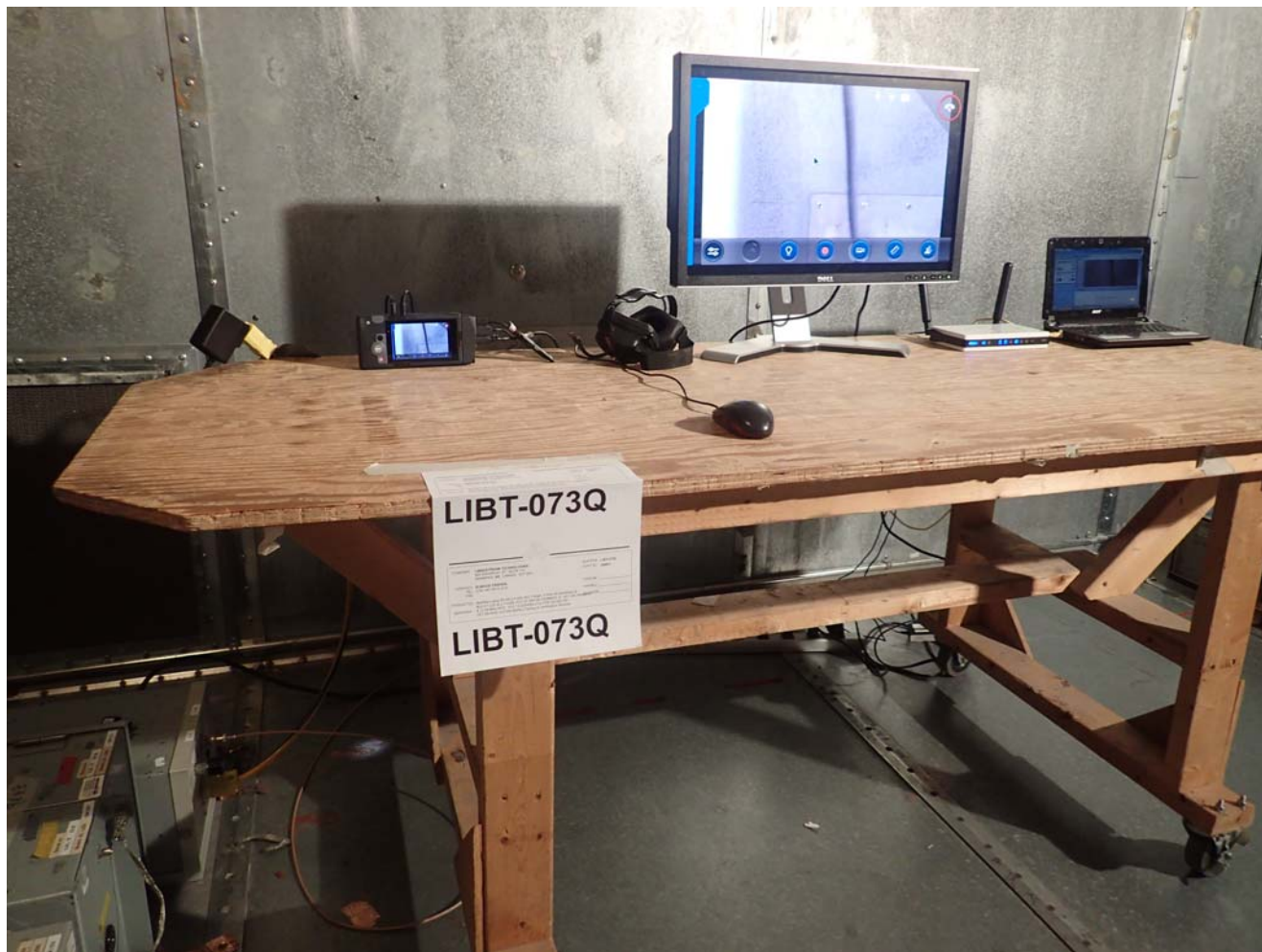
Power Line Conducted Emission (without aluminum shield)
