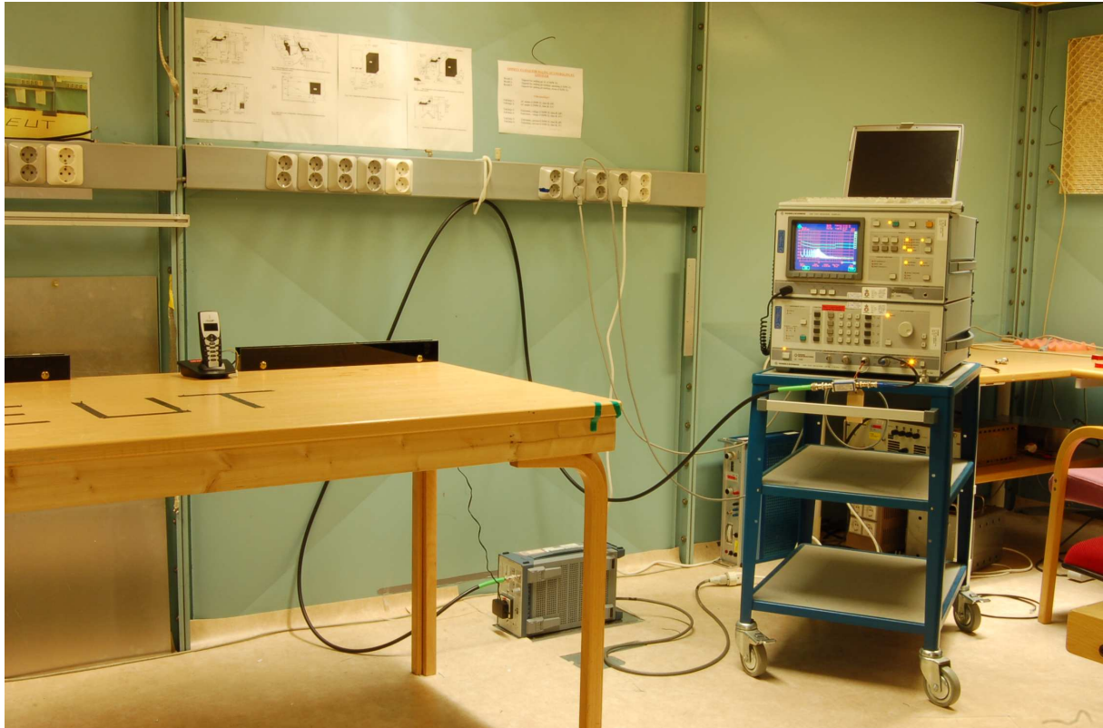
CT7141H-US – Power line Conducted Emissions Test
