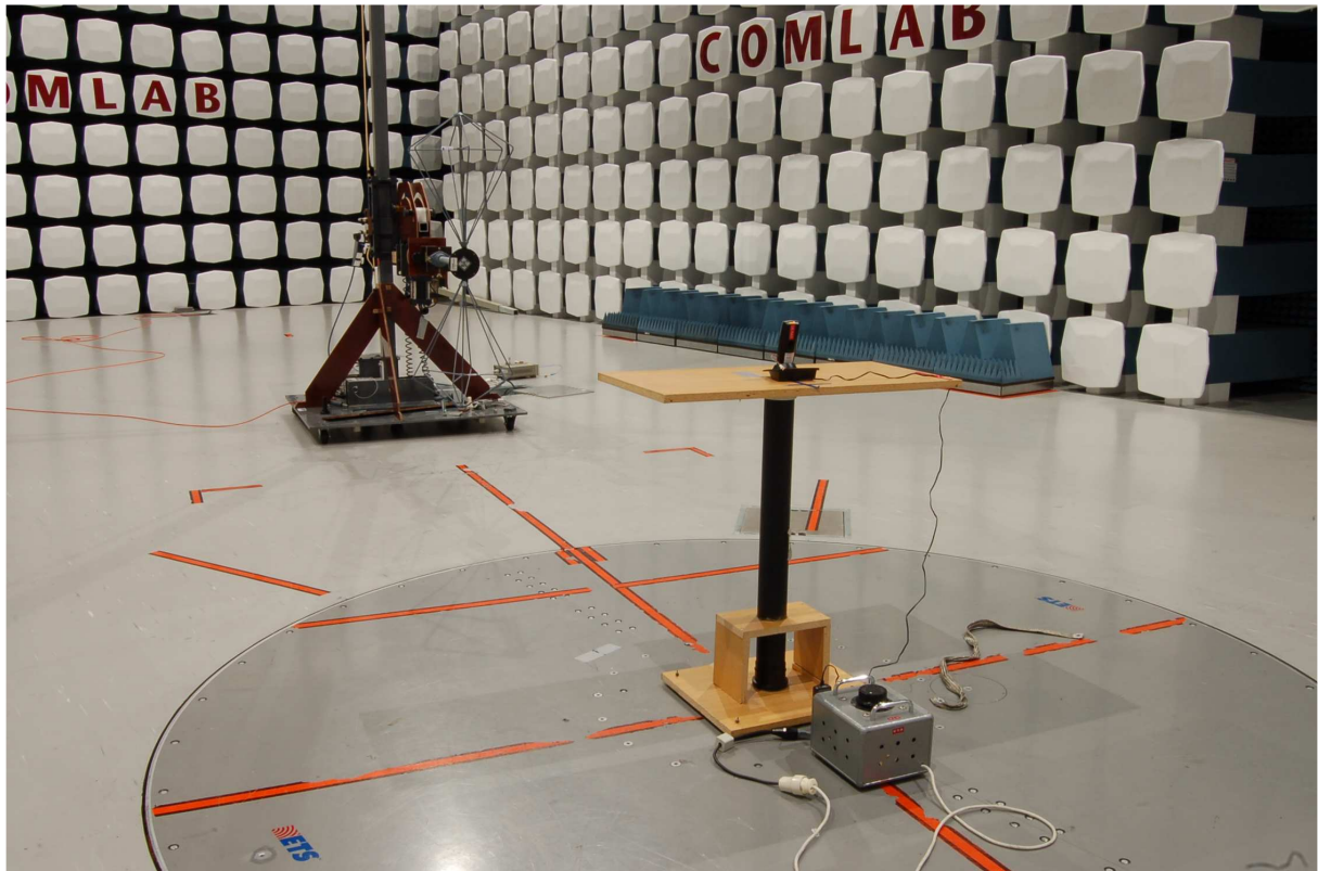
CT7141H-US - Radiated emission 30 - 200 MHz
