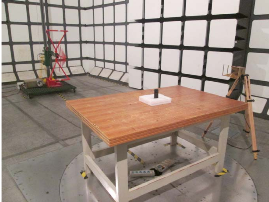
Radiated Emissions View (Below 1 GHz)
