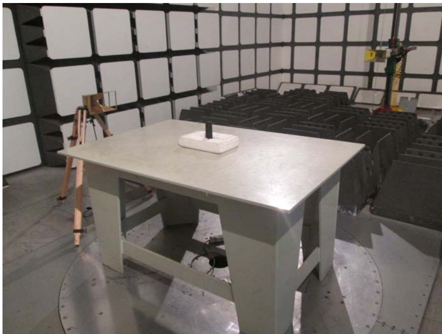
Radiated Emissions View (Above 1 GHz)
