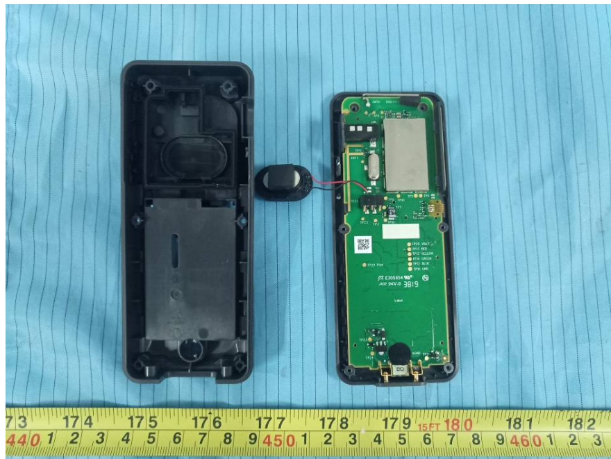
EUT – Cover off View 2
