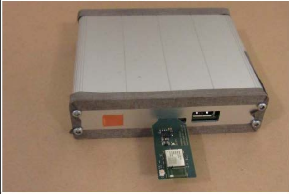
Processor board radiated, front view
