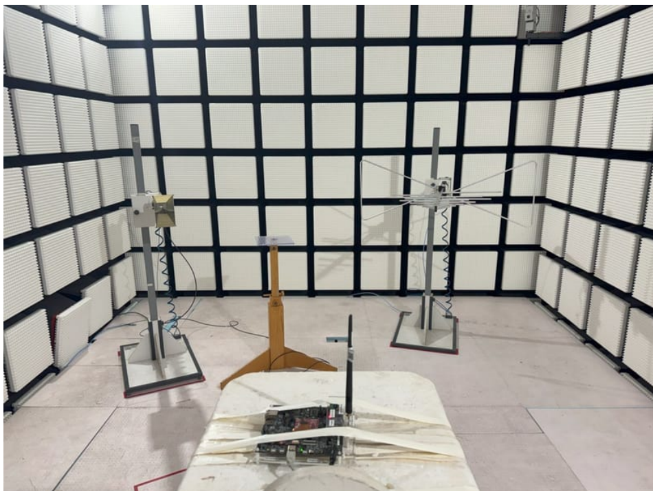
Photo 7: RSE set-up > 1 GHz with Taoglas antenna
