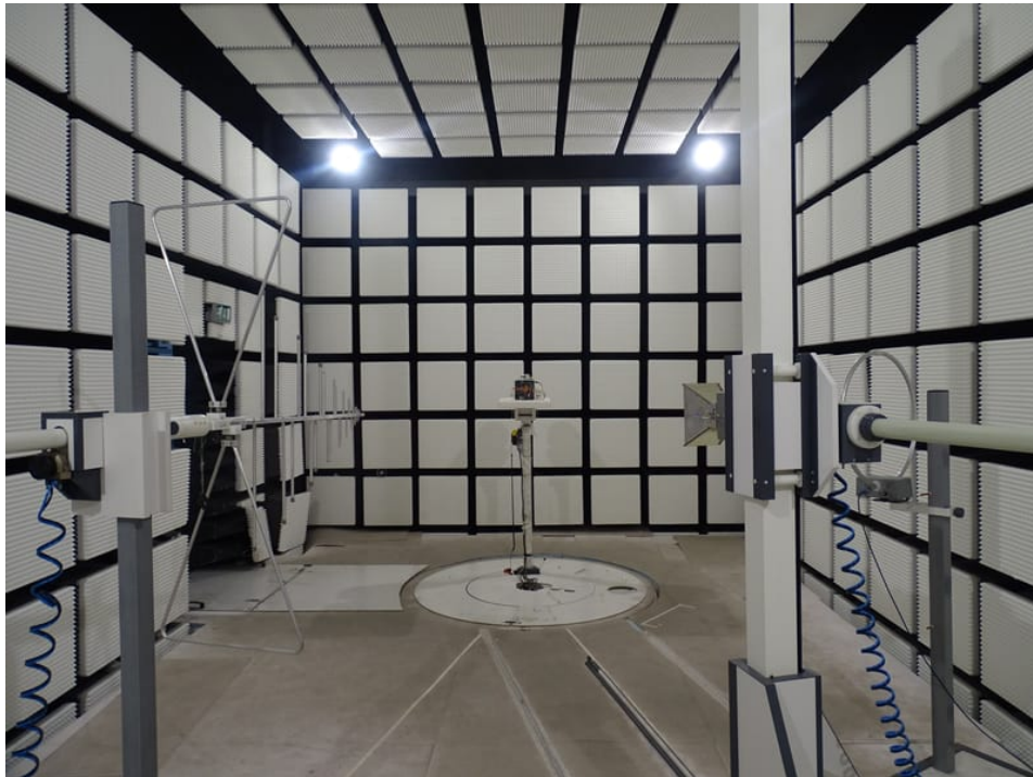
Photo 11: RSE set-up > 1 GHz with 2J antenna
