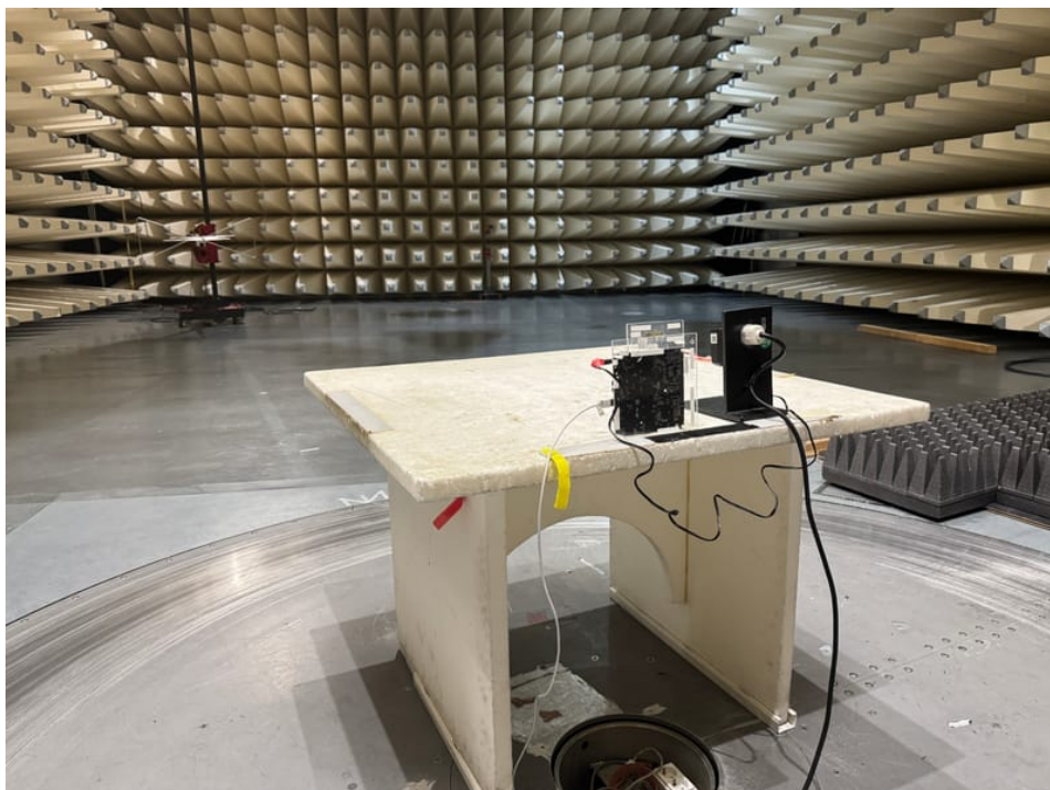
Photo 4: RSE set-up < 1 GHz with 2J antenna
