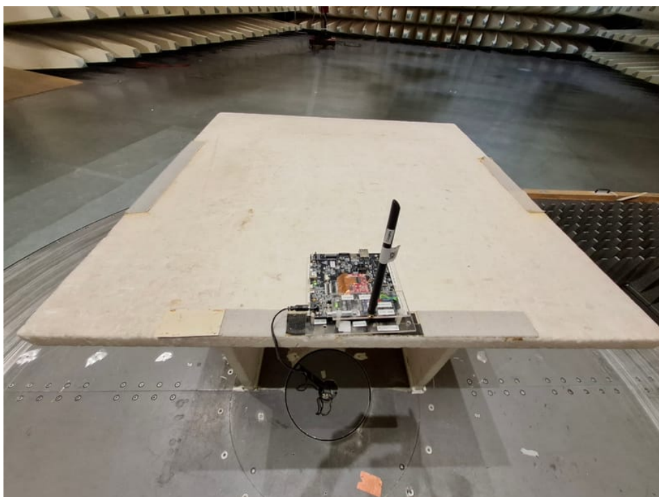
Photo 2: RSE set-up < 1 GHz with Taoglas antenna
