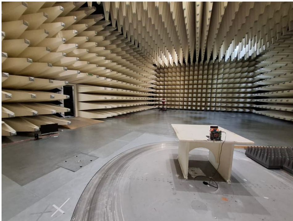
Photo 1: RSE set-up < 1 GHz with chip antenna
