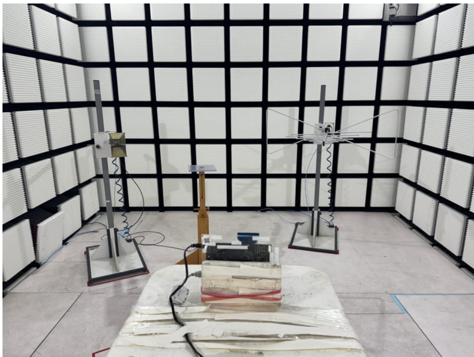
Photo 4: RSE set-up > 1 GHz with chip antenna
