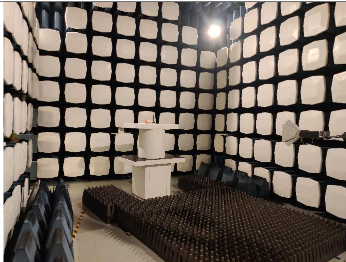
Picture 10, Radiated Spurious Emissions, common setup, TX, 1 – 26 GHz
