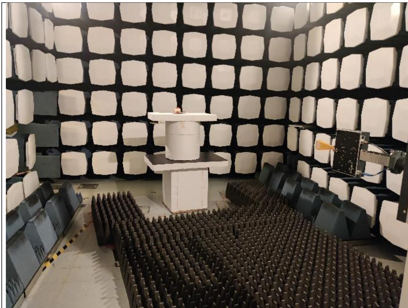
Picture 11, Radiated Spurious Emissions, common setup, TX, 26 – 40 GHz
