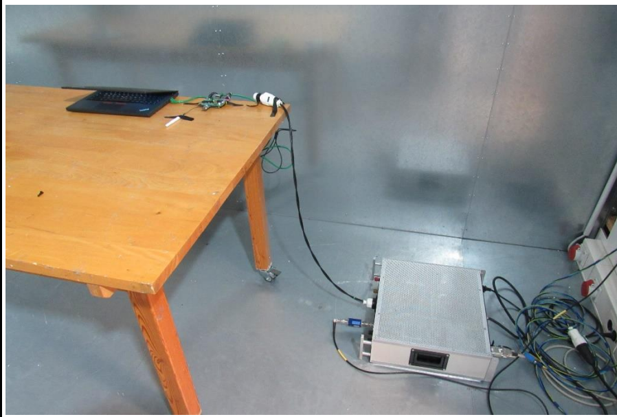
Setup for measurements 150 kHz - 30 MHz
