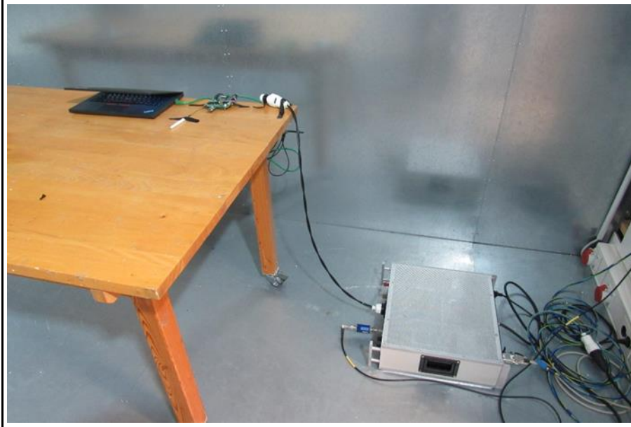
Test setup A - conducted measurement
