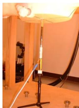
2450MHz System performance check setup
