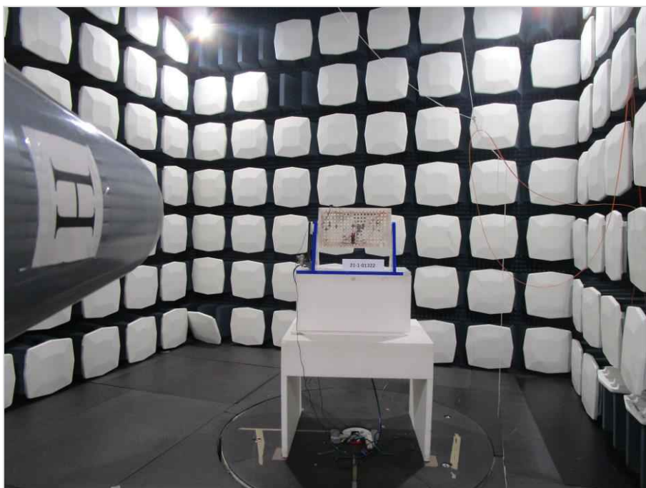
Photograph 4: EUT Test Setup in the fully anechoic chamber, Electric Field Strength
