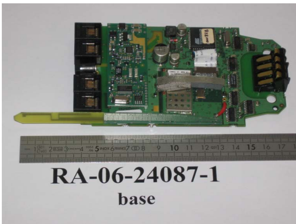
Printed circuit of the base with antenna
