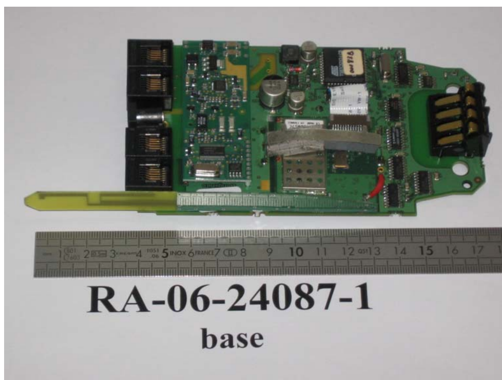
Printed circuit of the base with antenna
