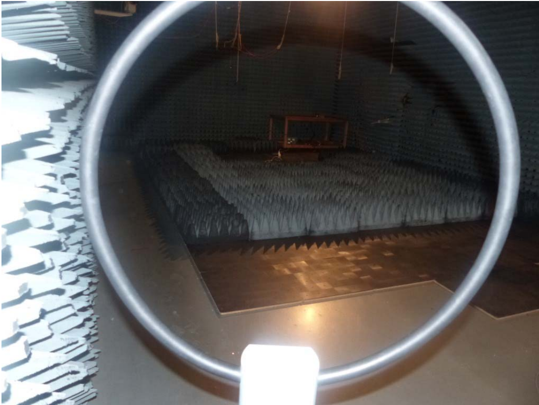
Photo 1: Radiated test setup for H-Field
