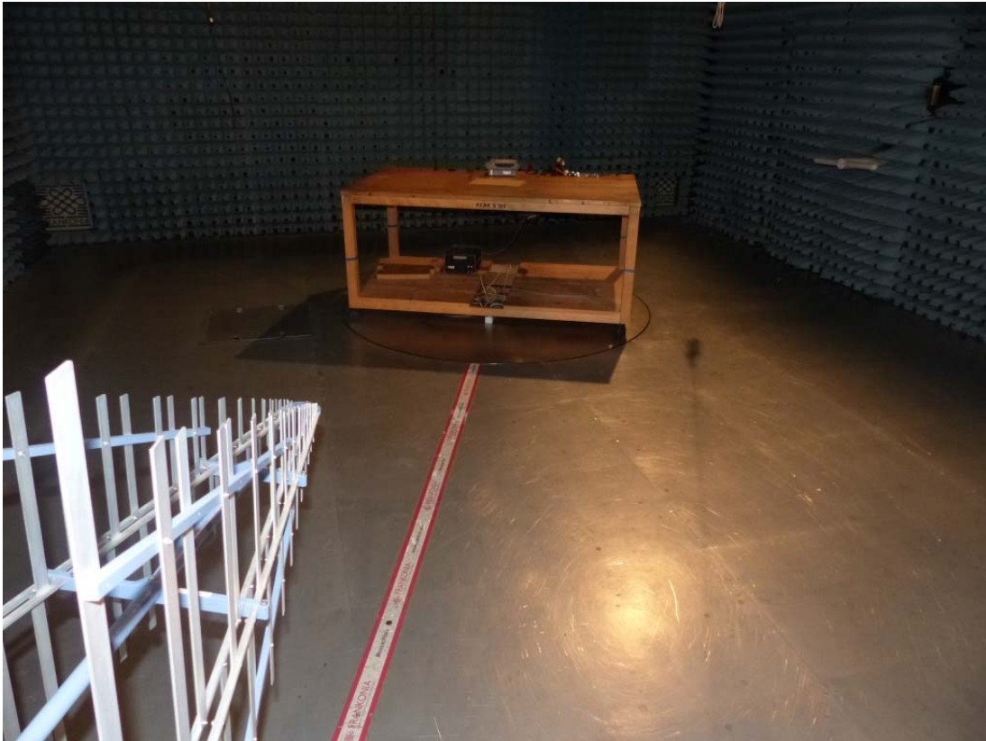
Photo 3: Radiated test setup for 30MHz – 1 GHz.
