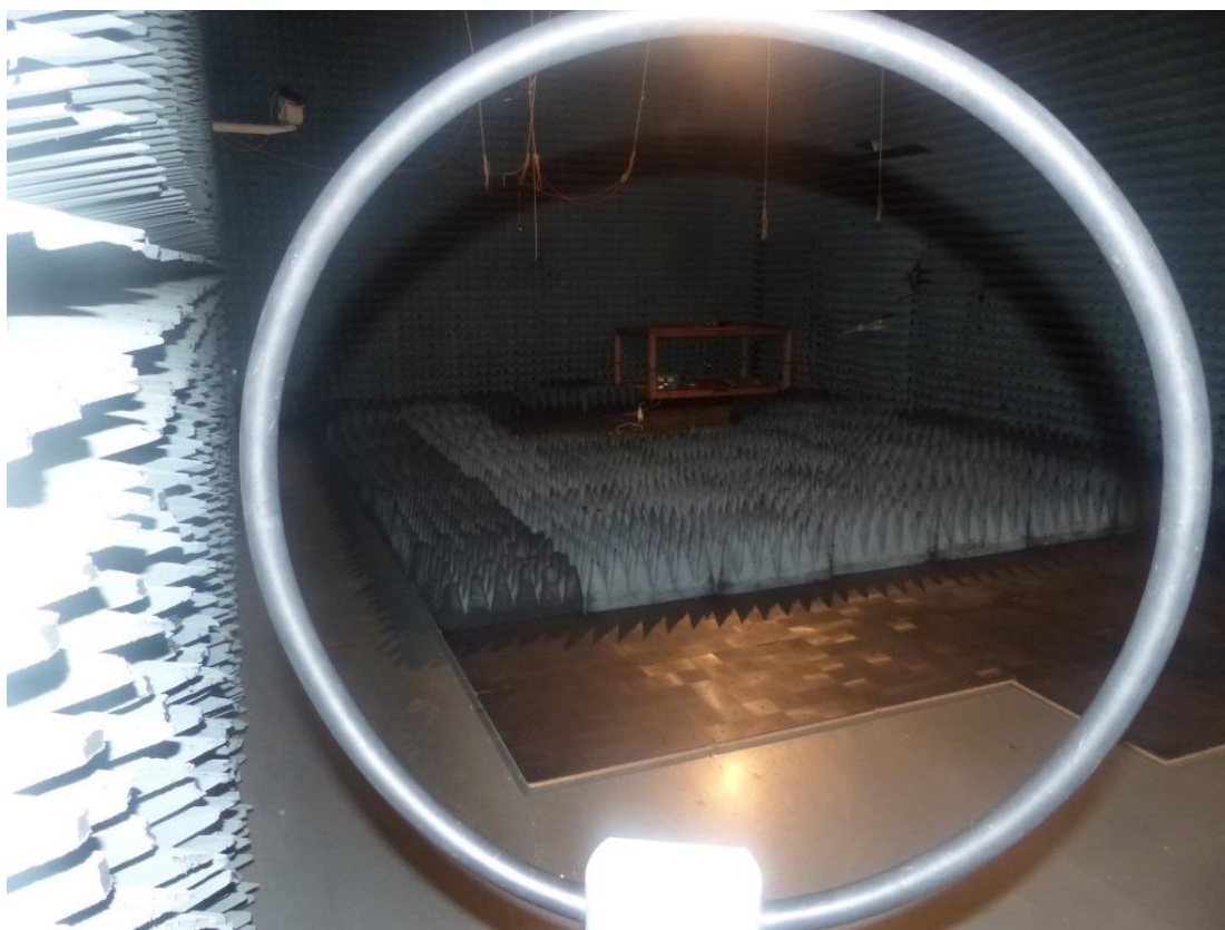
Photo 1: Radiated test setup for H-Field
