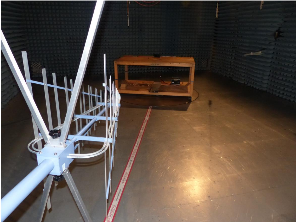
Photo 3: Radiated test setup for 30MHz – 1 GHz.
