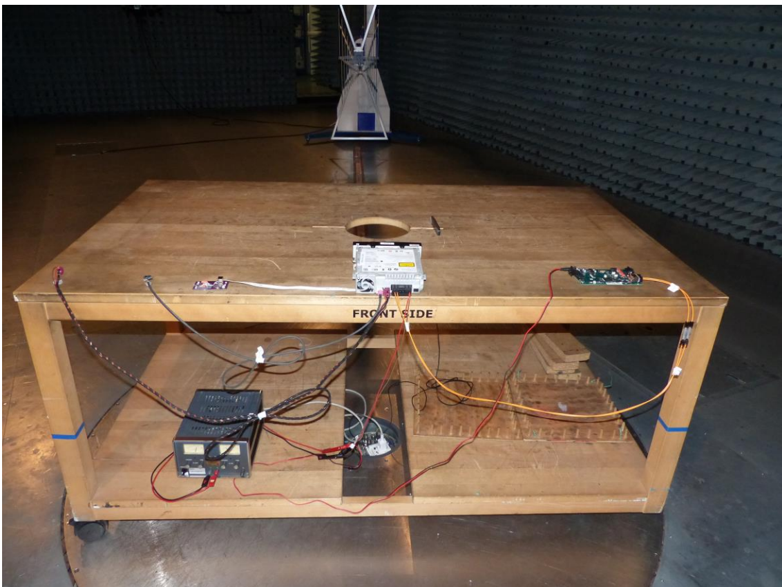
Photo 4: Radiated test setup for 30MHz – 1 GHz.
