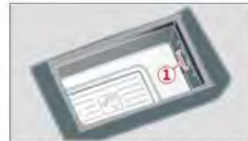
Fig. 173 Storage compartment under the center armrest: Principle of operation: Audi phone box with connections
