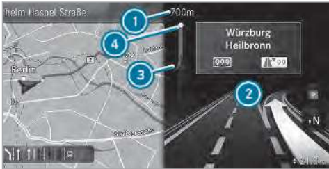
Example: 3D image of the upcoming change of direction ① Current distance to the change of direction ② Changing direction ③ Current vehicle position ④ Manoeuvre point
