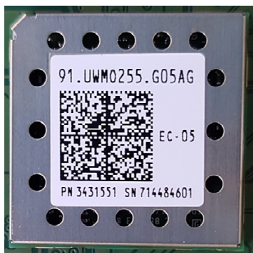
BT/WLAN-Module with shielding plate (20x20mm)
