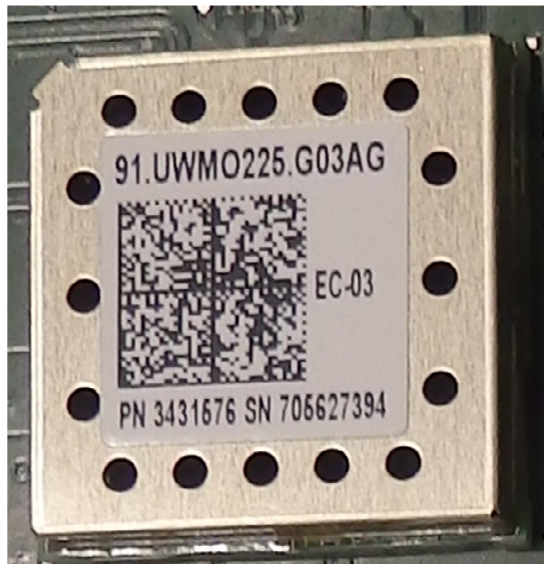
BT/WLAN-Module with shielding plate (20x20mm)
