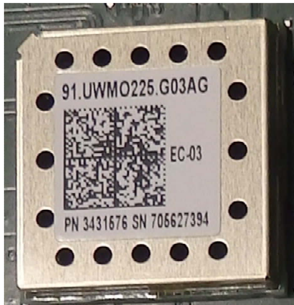
BT/WLAN-Mod with shielding plate (20x20mm)
