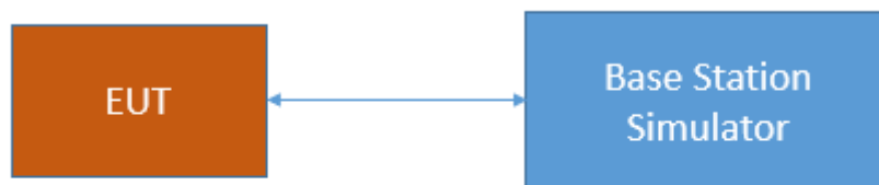
Test Setup FCC Part 22/24/27/90 Cellular; Frequency stability
