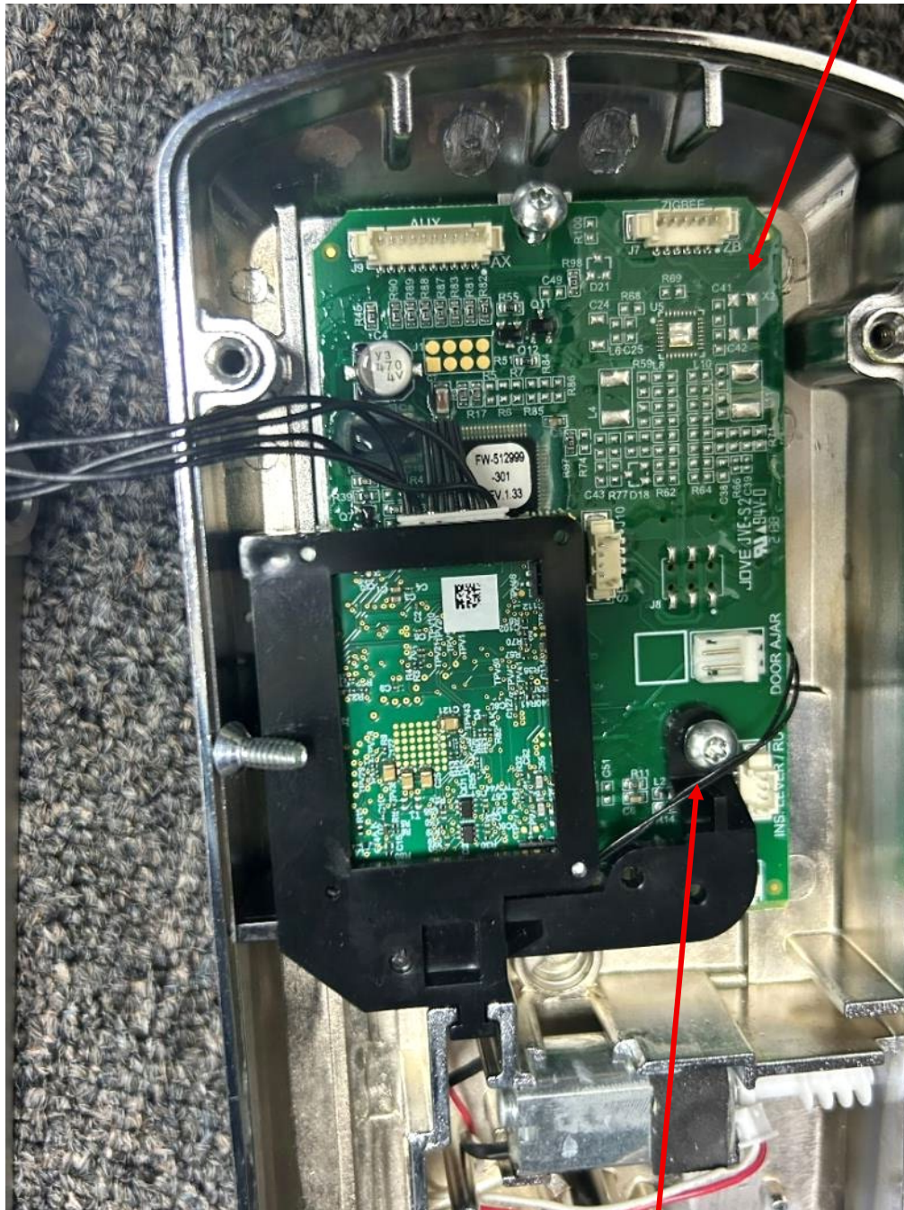
E7900 Host PCB and CSM-200 Module HF Antenna Connector Wire to HF Antenna
