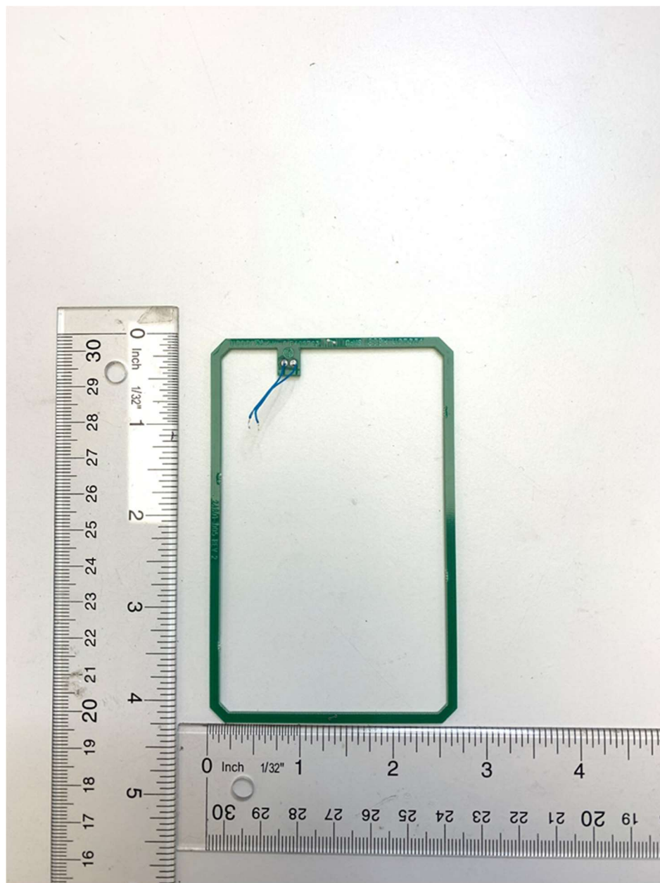
13.56MHz Coil Board - Farpointe Data, Inc. Confidential & Proprietary Information
