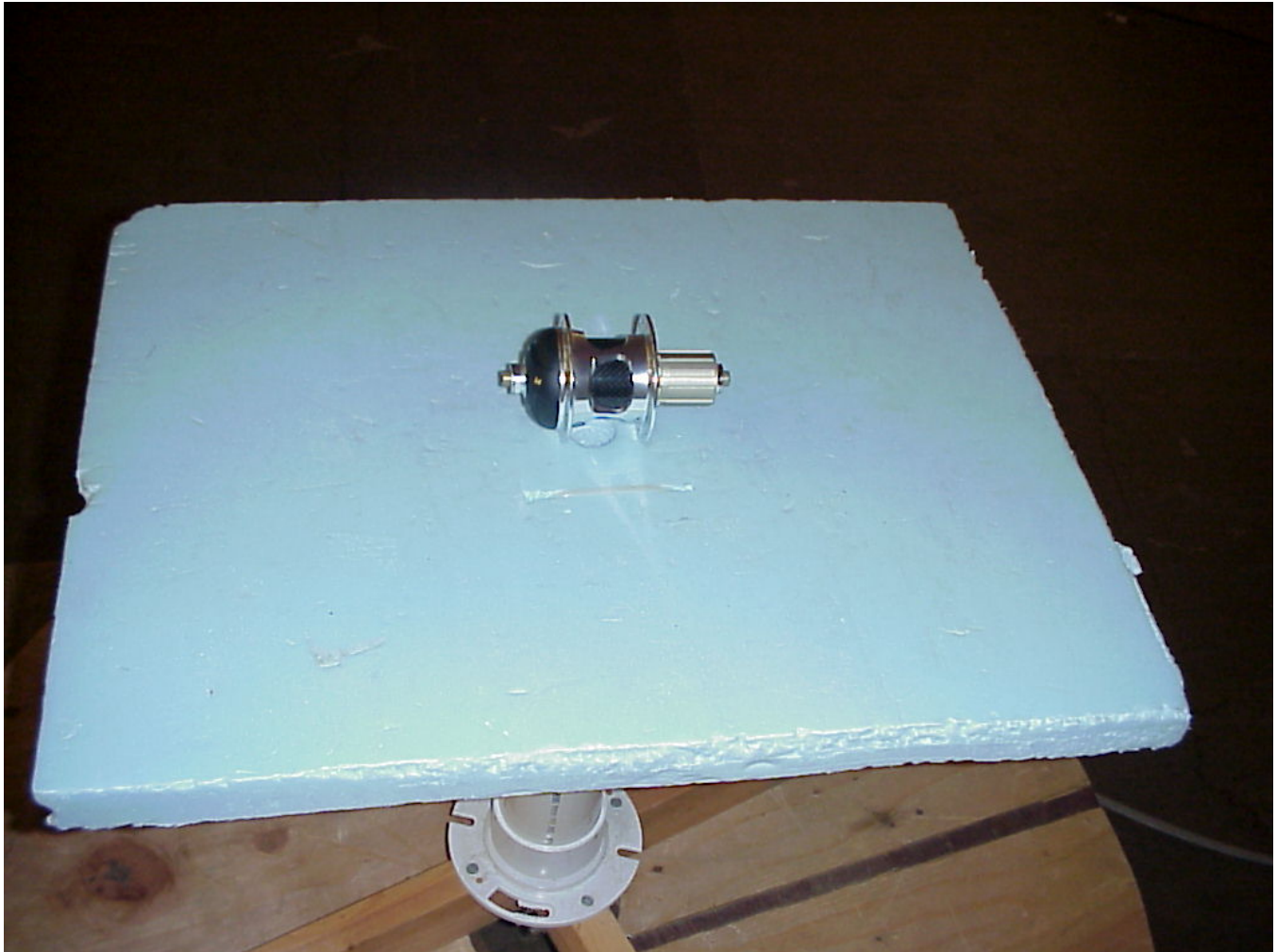
HUB TRANSMITTER CLOSE UP
