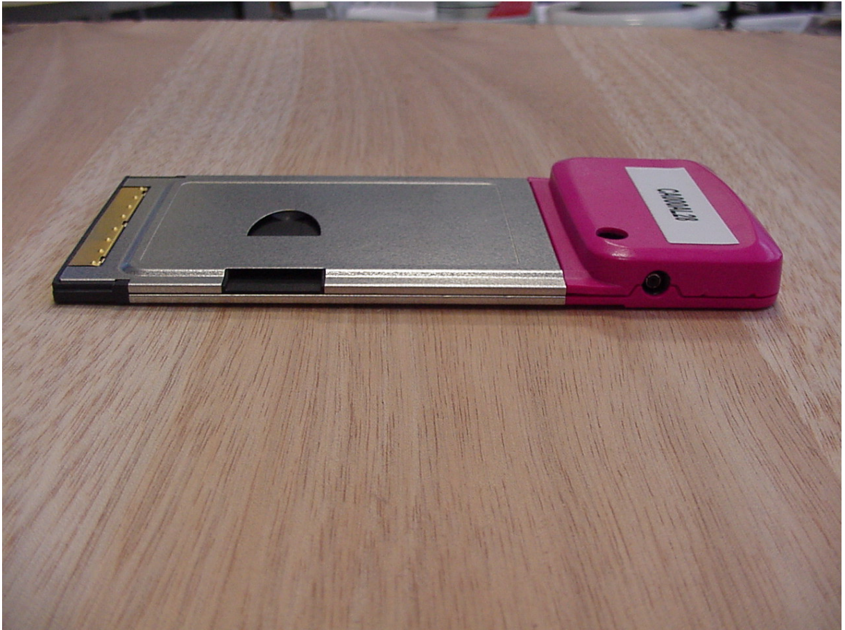
Photo 3: EUT (left side with SIM card holder and temporary antenna connector which was not used for testing)
