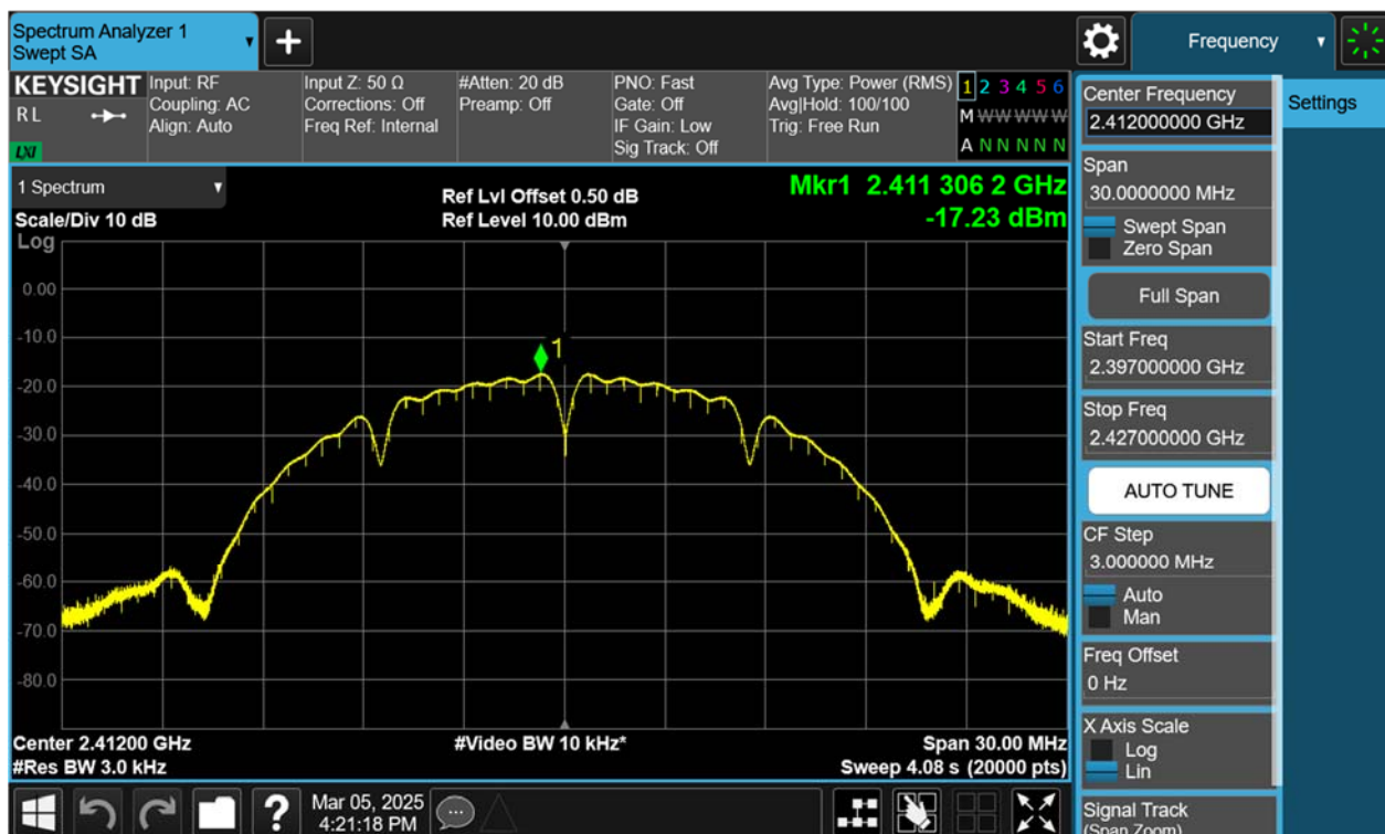
Figure 14: Power Spectral Density, 802.11b, 2437MHz
