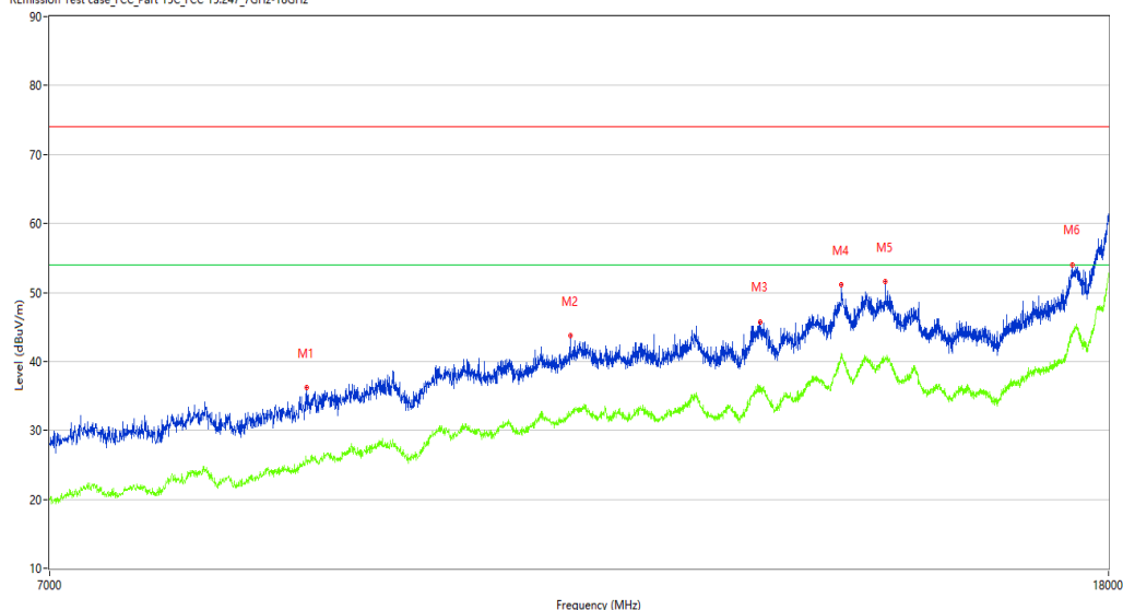
R Emission Test case_FCC_Part 15C_FCC 15.247_7GHz-18GHz
