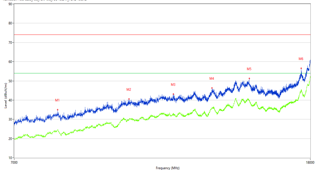
R Emission Test case_FCC_Part 15C_FCC 15.247_7GHz-18GHz
