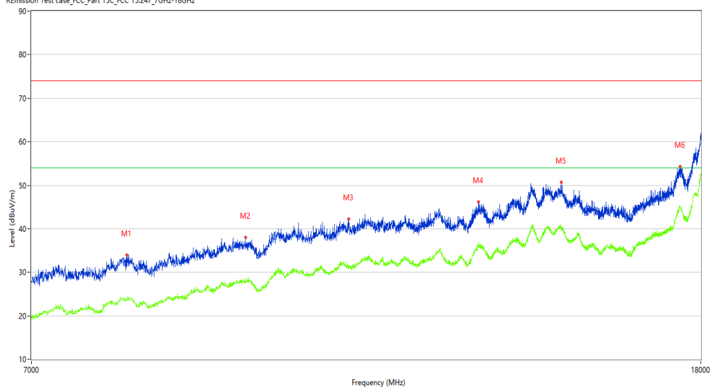
REmission Test case_FCC_Part 15C_FCC 15.247_7GHz-18GHz
