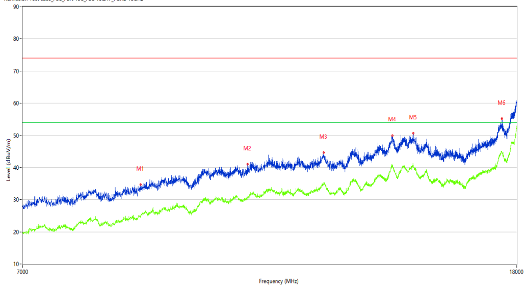
REmission Test case_FCC_Part 15C_FCC 15.247_7GHz-18GHz
