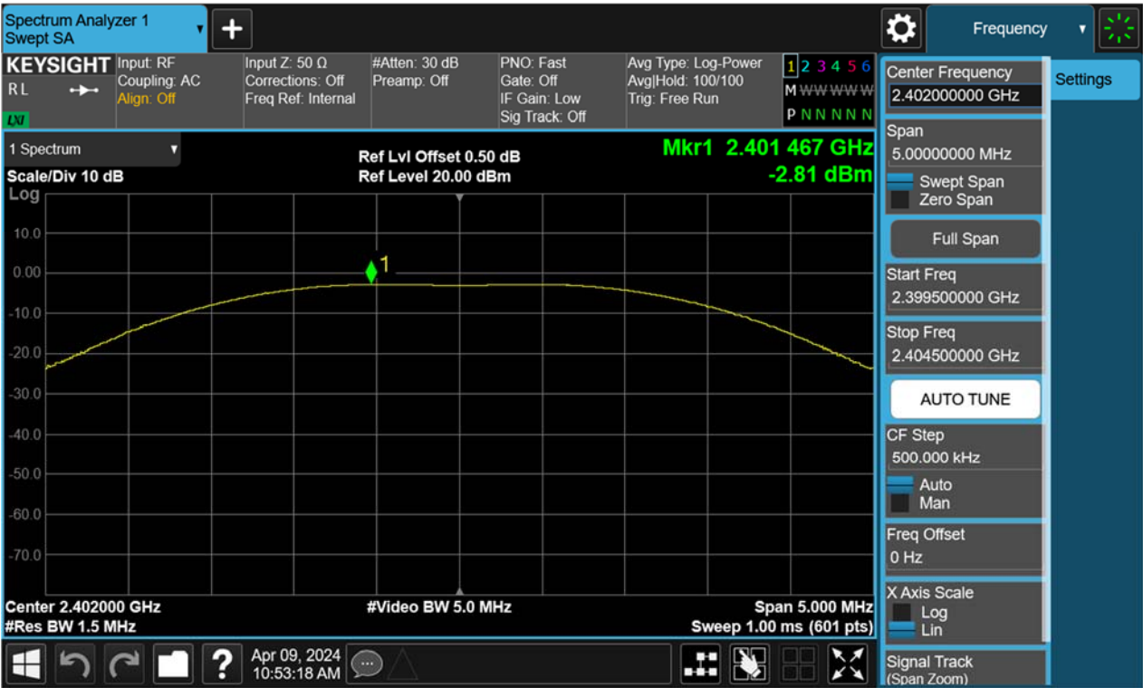
Figure 4: Peak Output Power, 2402MHz, BLE-2Mbps
