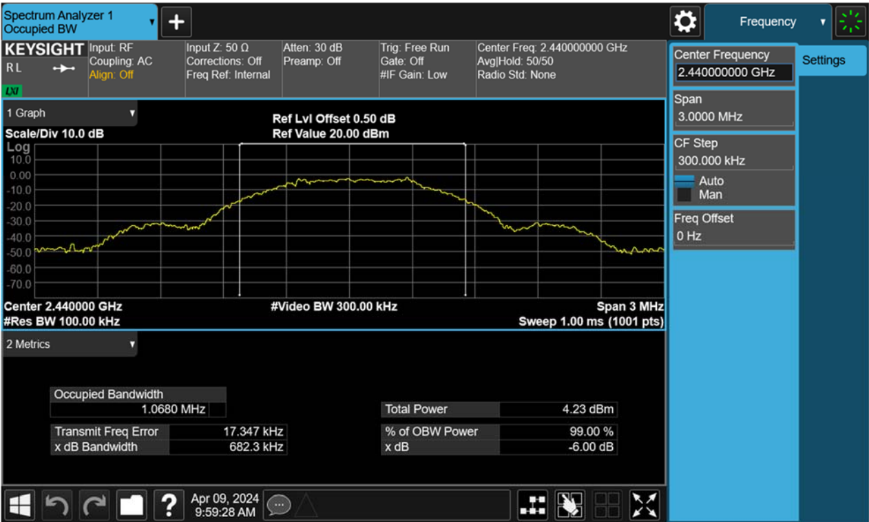
Figure 26: 6dB Bandwidth, 2440MHz, BLE-1Mbps
