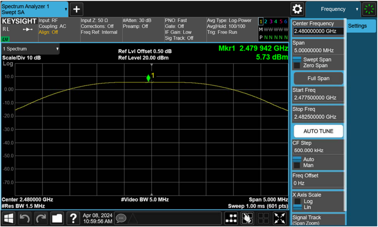
Figure 18: Peak Output Power, 2480MHz, BLE-2Mbps
