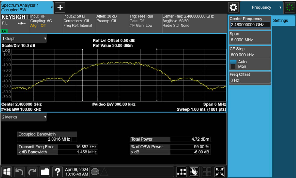
Figure 30: 6dB Bandwidth, 2480MHz, BLE-2Mbps
