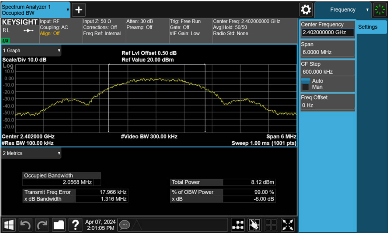
Figure 28: 6dB Bandwidth, 2402MHz, BLE-2Mbps
