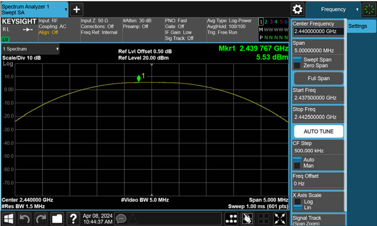
Figure 14: Peak Output Power, 2440MHz, BLE-1Mbps
