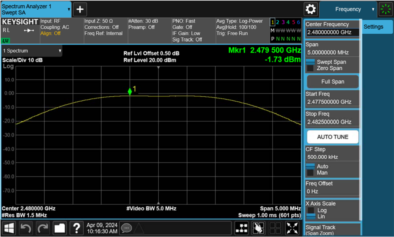
Figure 12: Peak Output Power, 2480MHz, BLE-2Mbps
