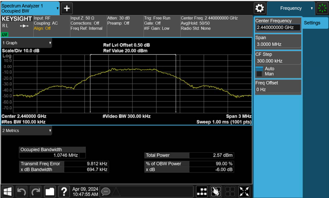
Figure 20: 6dB Bandwidth, 2440MHz, BLE-1Mbps
