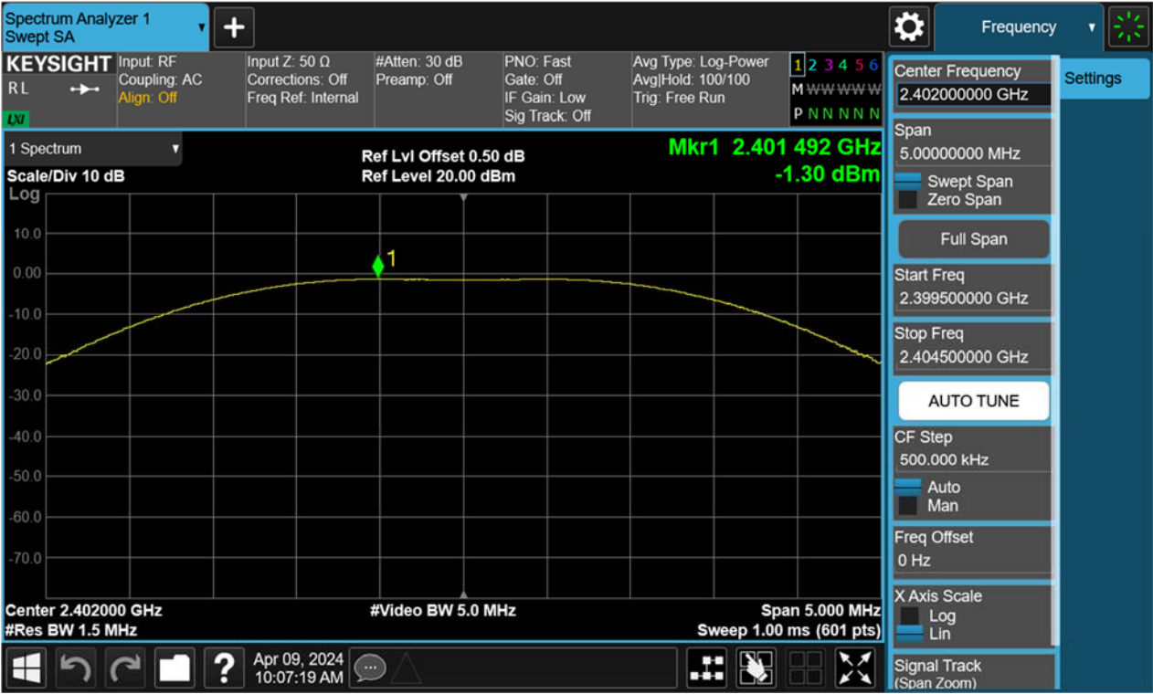
Figure 10: Peak Output Power, 2402MHz, BLE-2Mbps
