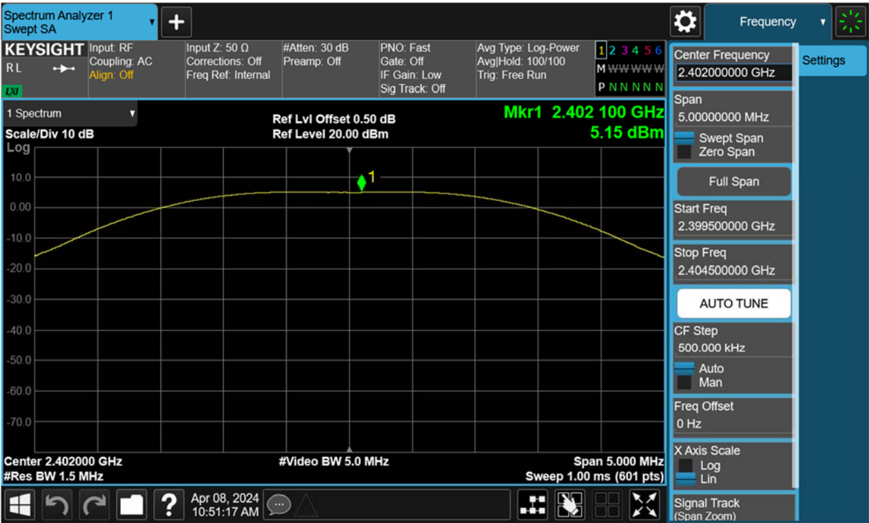
Figure 16: Peak Output Power, 2402MHz, BLE-2Mbps
