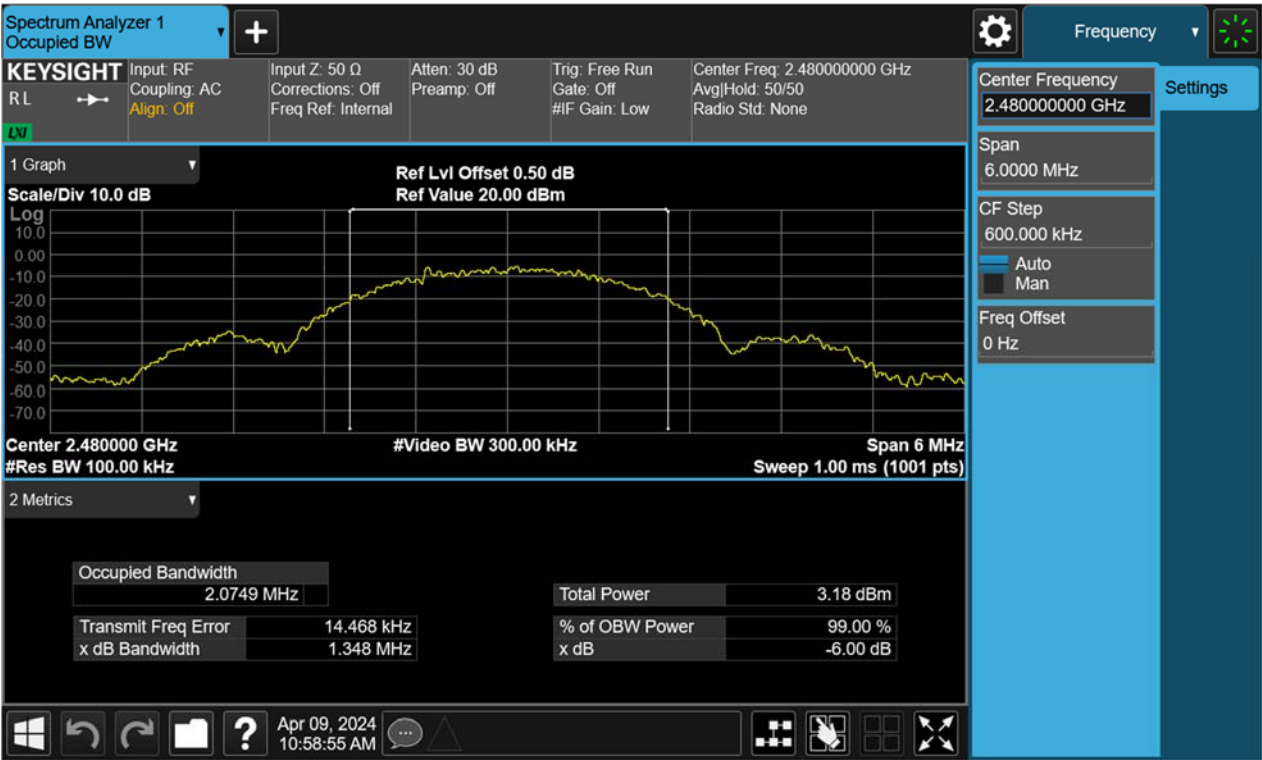
Figure 24: 6dB Bandwidth, 2480MHz, BLE-2Mbps
