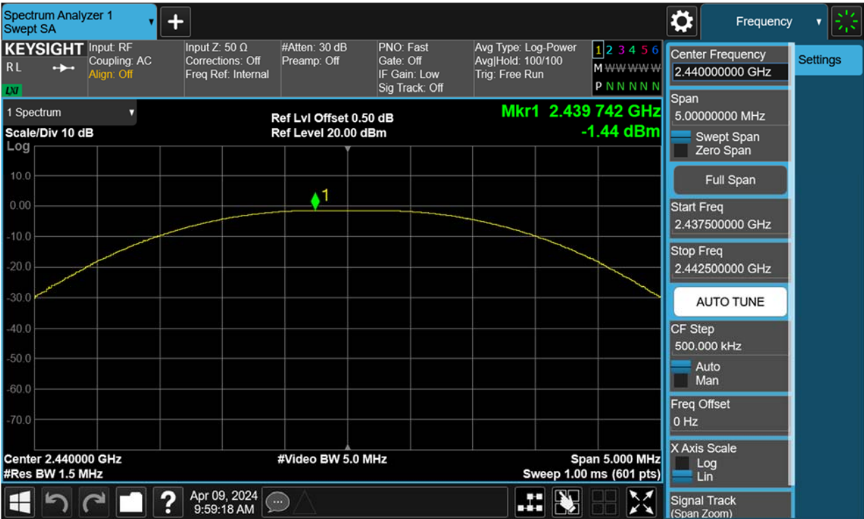
Figure 8: Peak Output Power, 2440MHz, BLE-1Mbps
