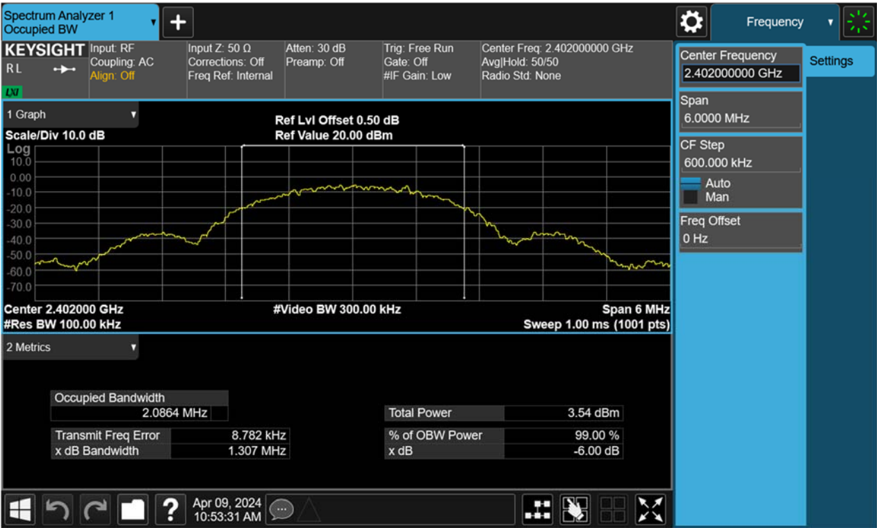
Figure 22: 6dB Bandwidth, 2402MHz, BLE-2Mbps
