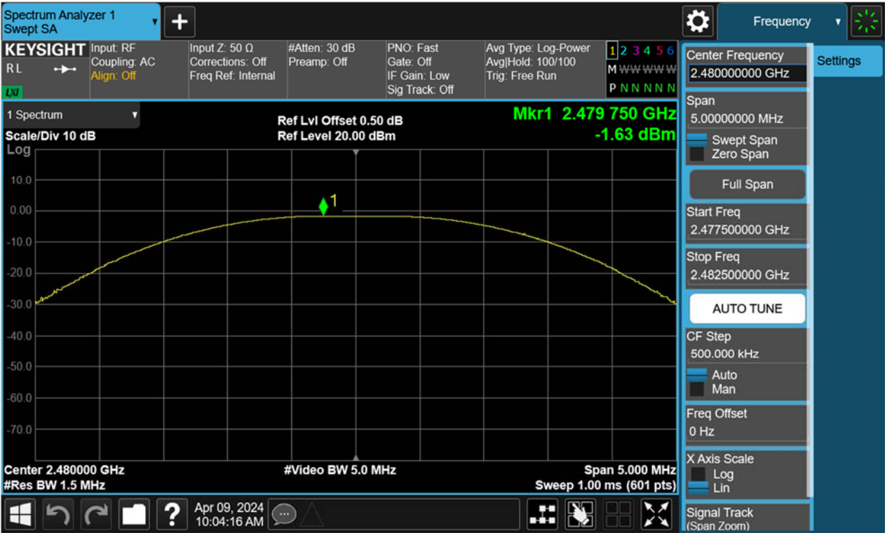
Figure 10: Peak Output Power, 2402MHz, BLE-2Mbps
