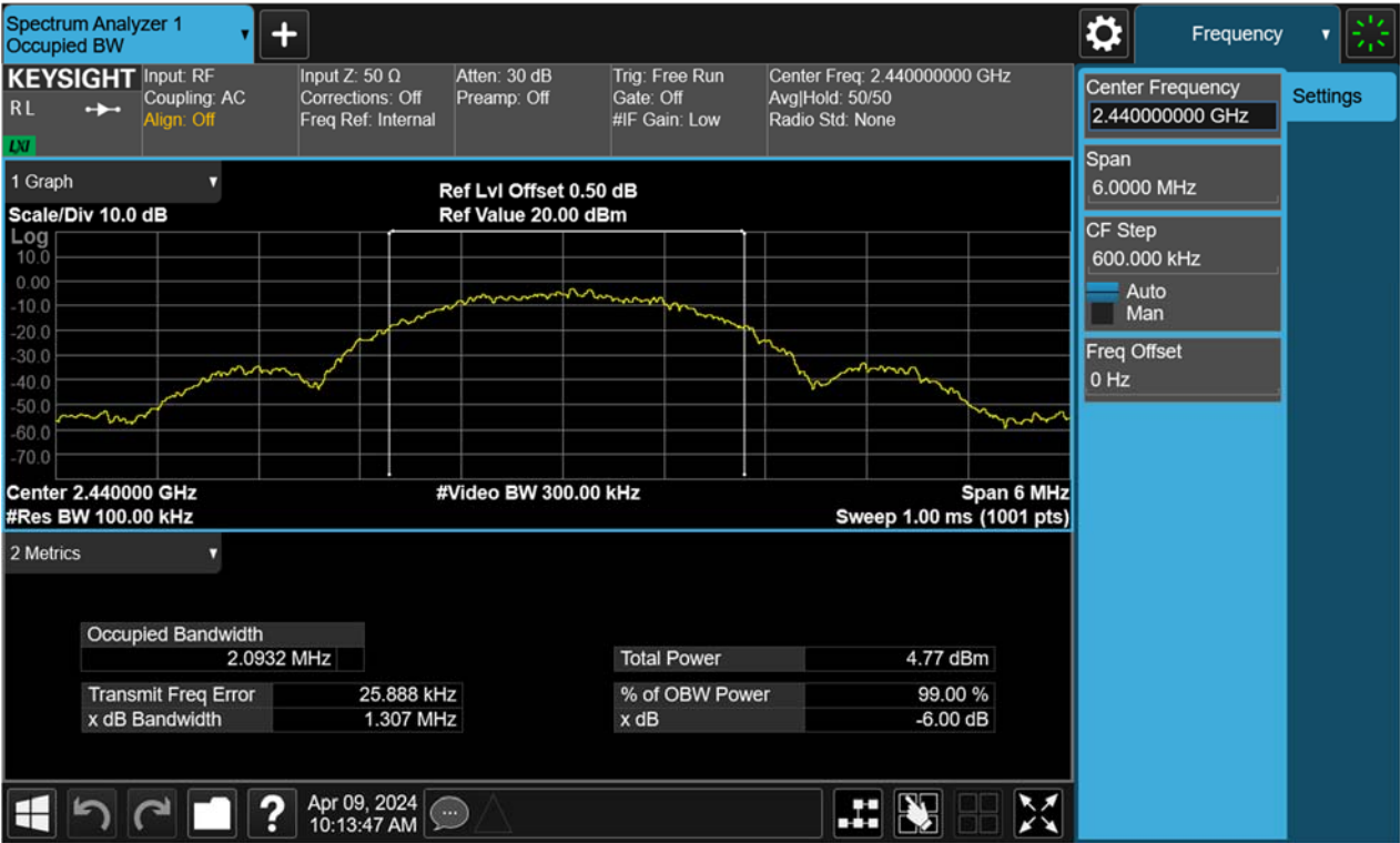
Figure 30: 6dB Bandwidth, 2480MHz, BLE-2Mbps
