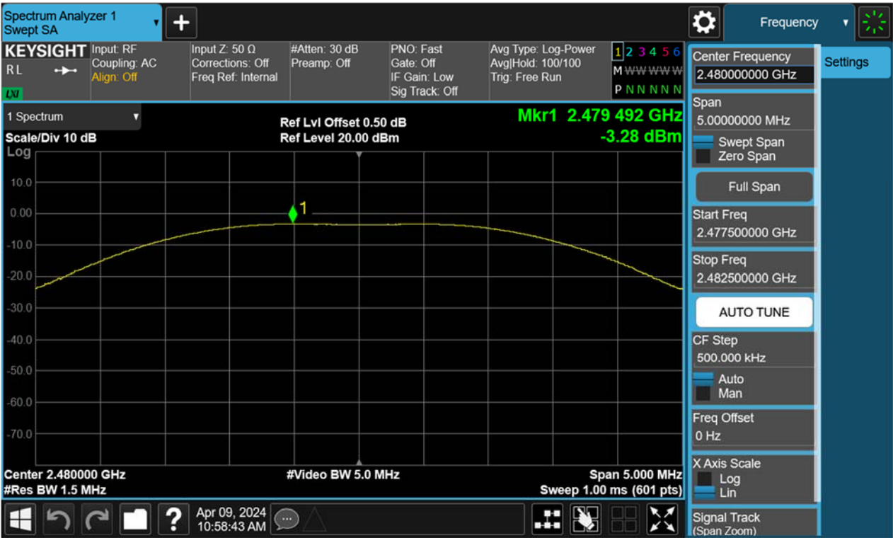
Figure 6: Peak Output Power, 2480MHz, BLE-2Mbps
