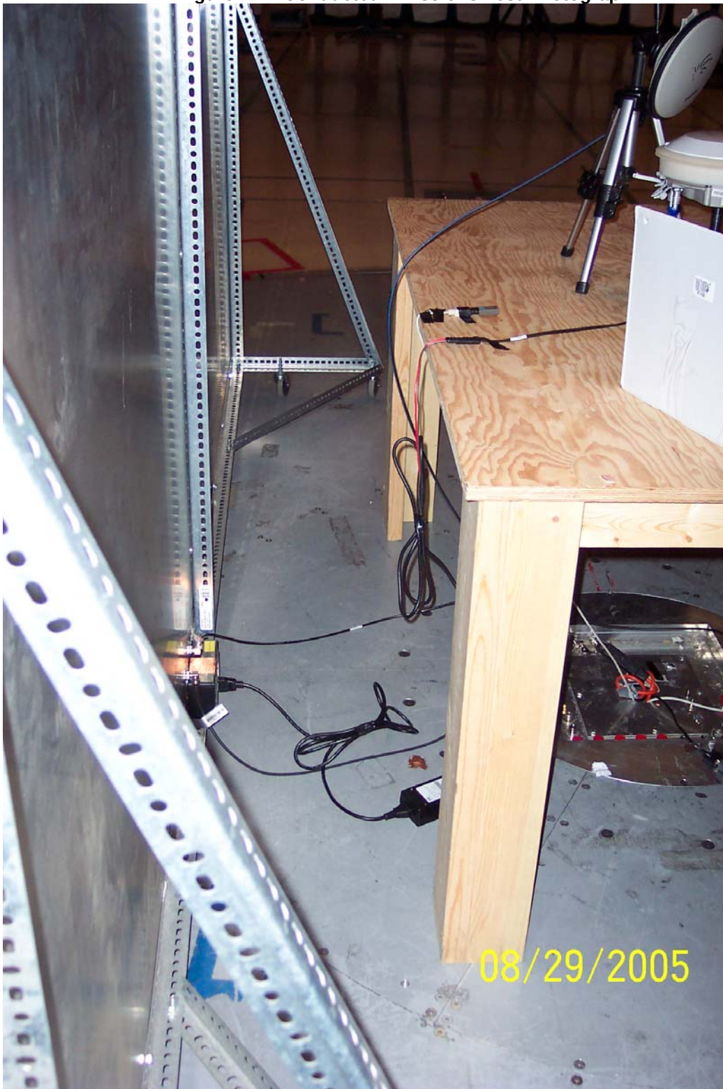
Figure 2 Conducted Emissions Test Photograph
