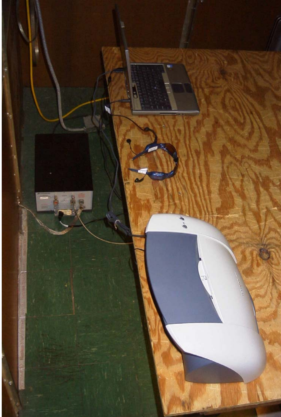
POWERLINE CONDUCTED EMISSIONS TEST SET UP PHOTO
