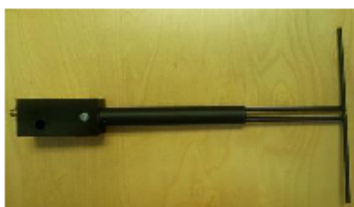
Figure 1 – MVG COMOSAR Validation Dipole
