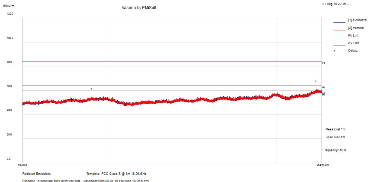
**26.5 GHz – 40 GHz Worst Case Scan at 1 meter***Worst Case Colocation, Radio 1-5 GHz Wi-Fi, Radio 2-5 GHz Wi-Fi and 2.4 GHz Classic Bluetooth*
