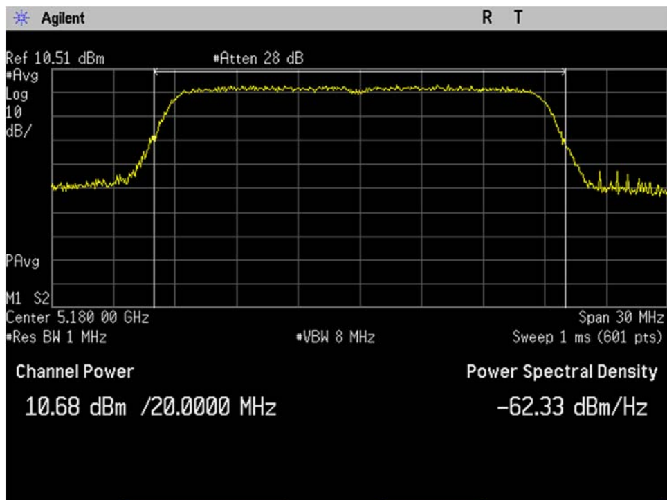
U-NII-1_5180MHz_Low Ch_36_20MHz BW_n-mode_Output Power_Port 2
