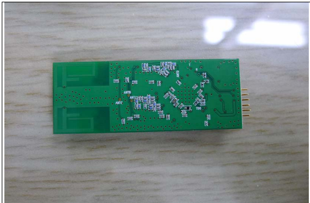
WLAN module board (Rear)
