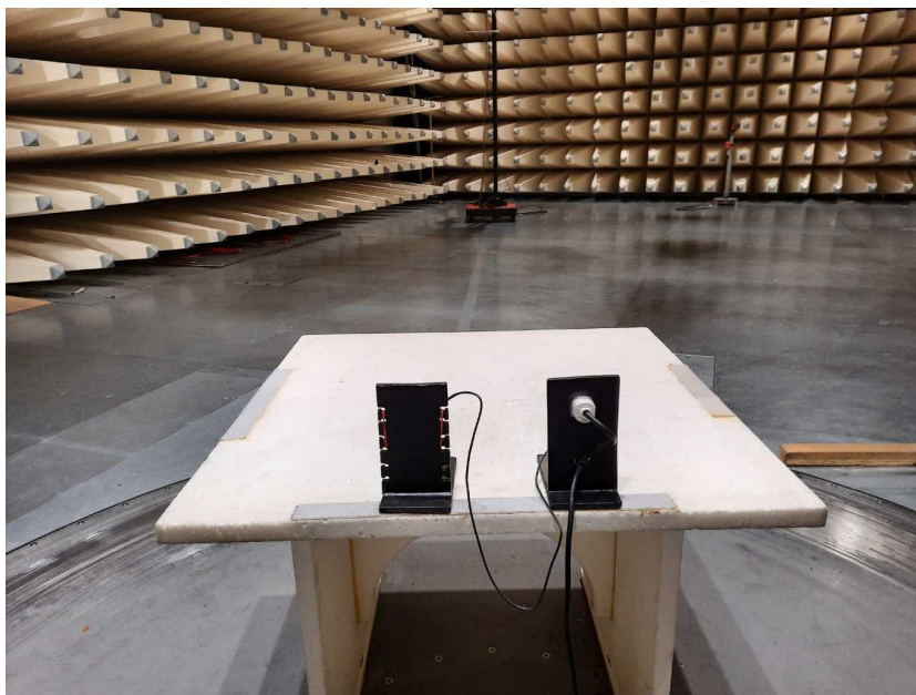
Photo 8: EUT at the semi-anechoic chamber
