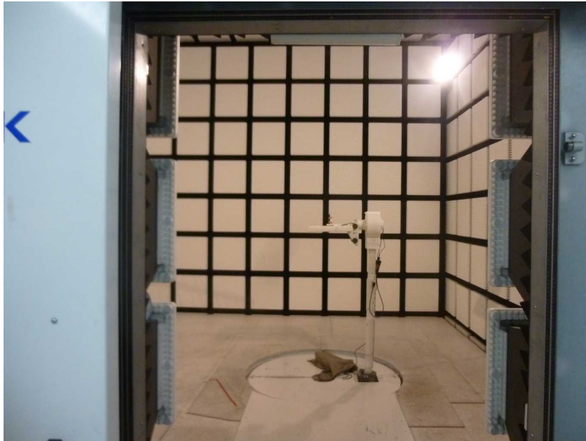
Photo 1: EUT at the anechoic chamber
