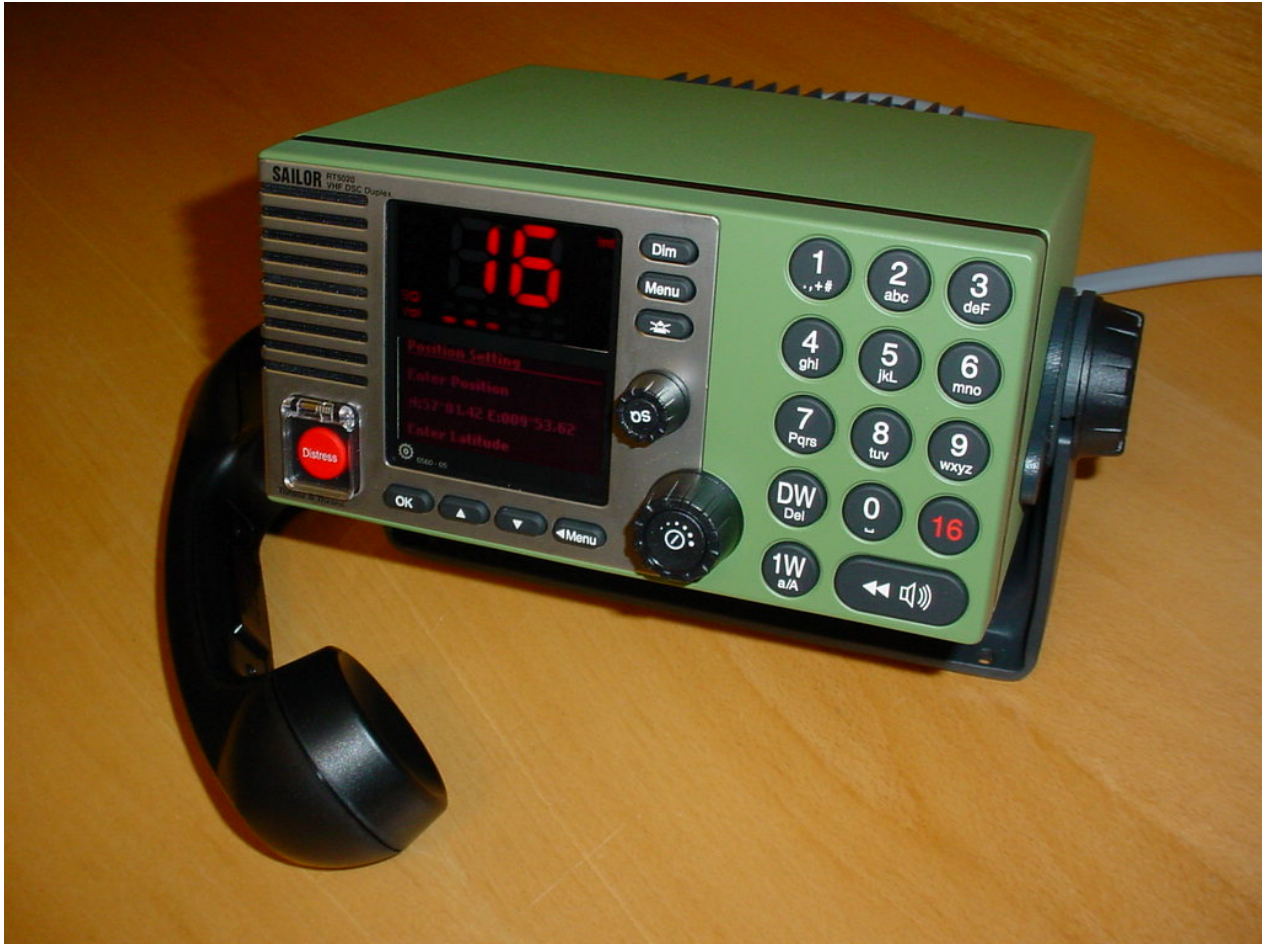
Front view with handset HS 5001. VHF mounted in bracket
