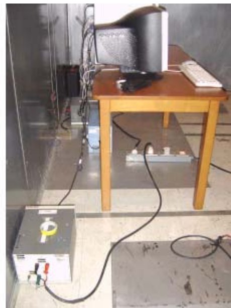
Figure 2 Test set up for conducted disturbance measurement
