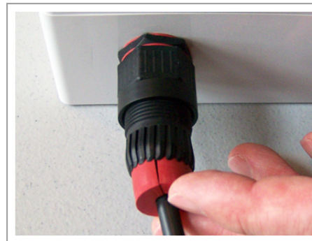
Figure 6.17. Slide cable bushing fully into connector B
