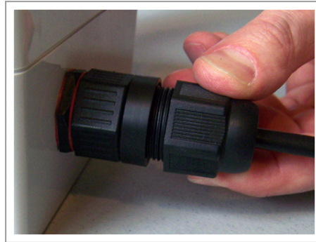
Figure 6.20. Thread connector A onto connector B and hand tighten
