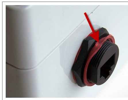
Figure 6.8. Replace damaged or used gaskets
