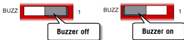
Figure 7.5. Setting the channel monitor buzzer with front-panel dip switch 1
