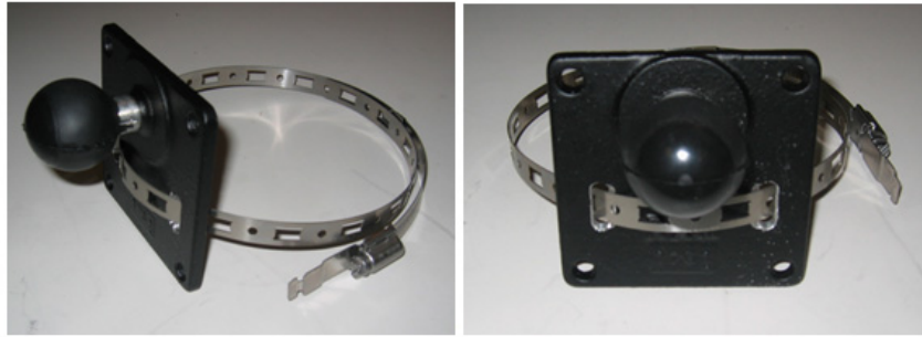
Figure 6.2. Clamp band threading through surface mounting ball plate
