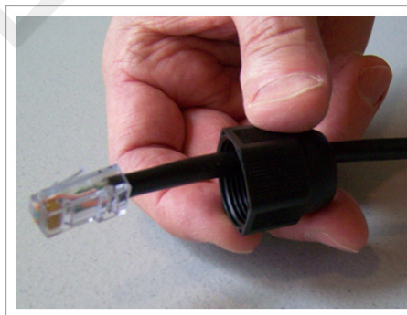
Figure 6.9. Thread cable through connector A
