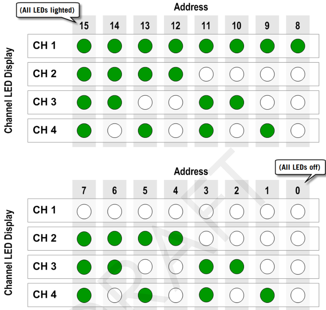
Figure A.1. Channel LED display / slot number combinations
