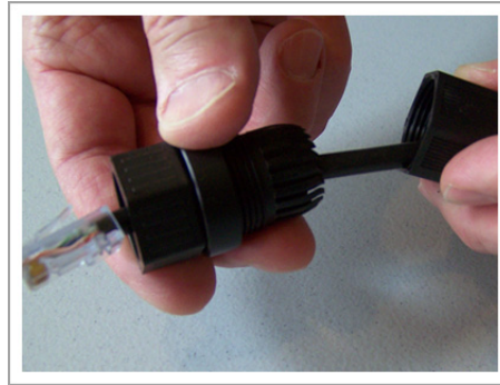
Figure 6.10. Thread cable through connector B
