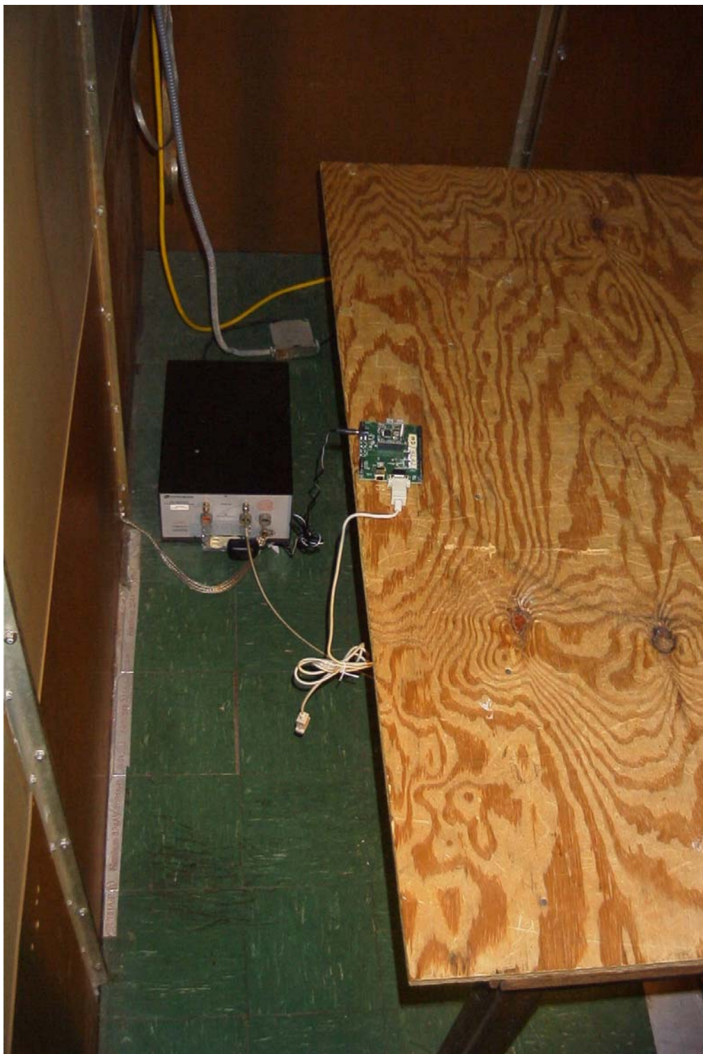
POWERLINE CONDUCTED EMISSIONS TEST SET UP PHOTO
