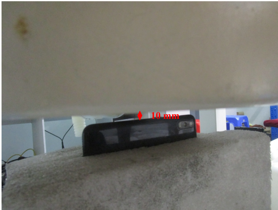
Body Bottom Setup Photo(10mm)
