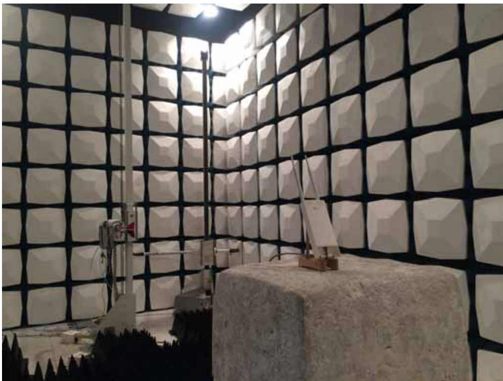
Description: Radiated Emission Test Setup for 1~18GHz
