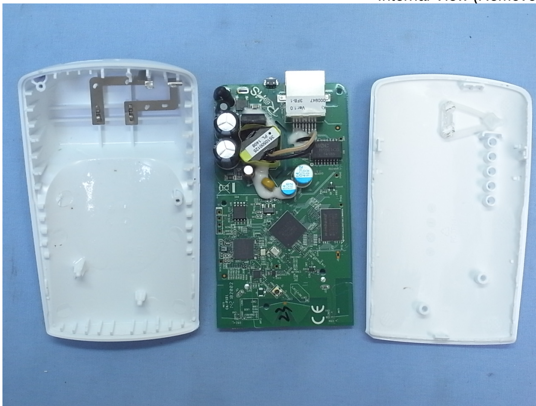
Figure 4 Internal View (Main Board, Front View)
